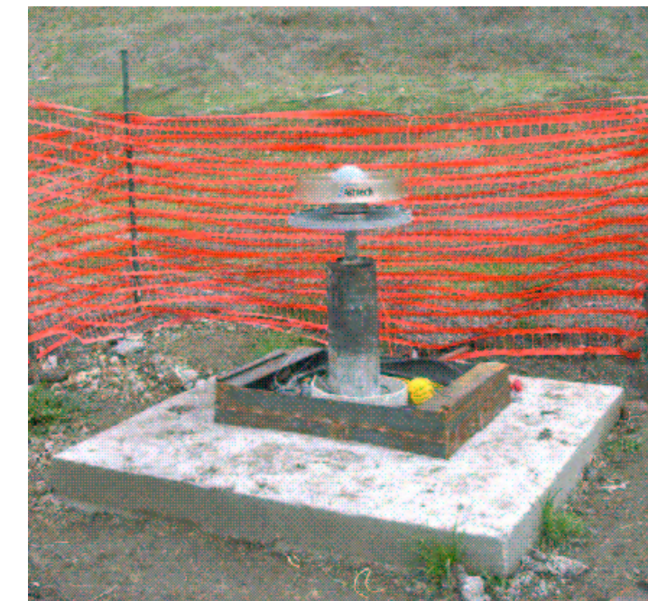
GPS antenna mounted on top of casing at OHLN. The final installation includes a SCIGN antenna dome and a steel protective shroud that envelopes the casing.
