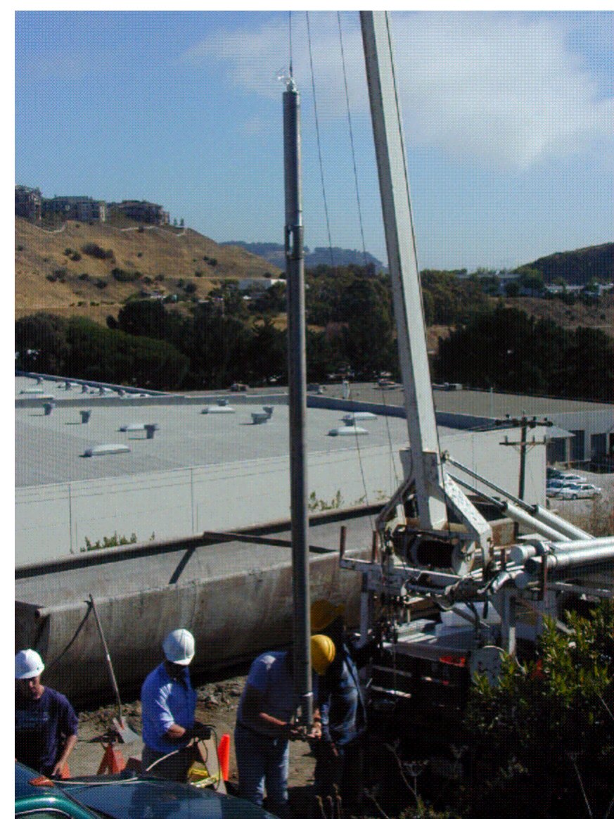
Deployment of the tensor strainmeter at San Bruno.
