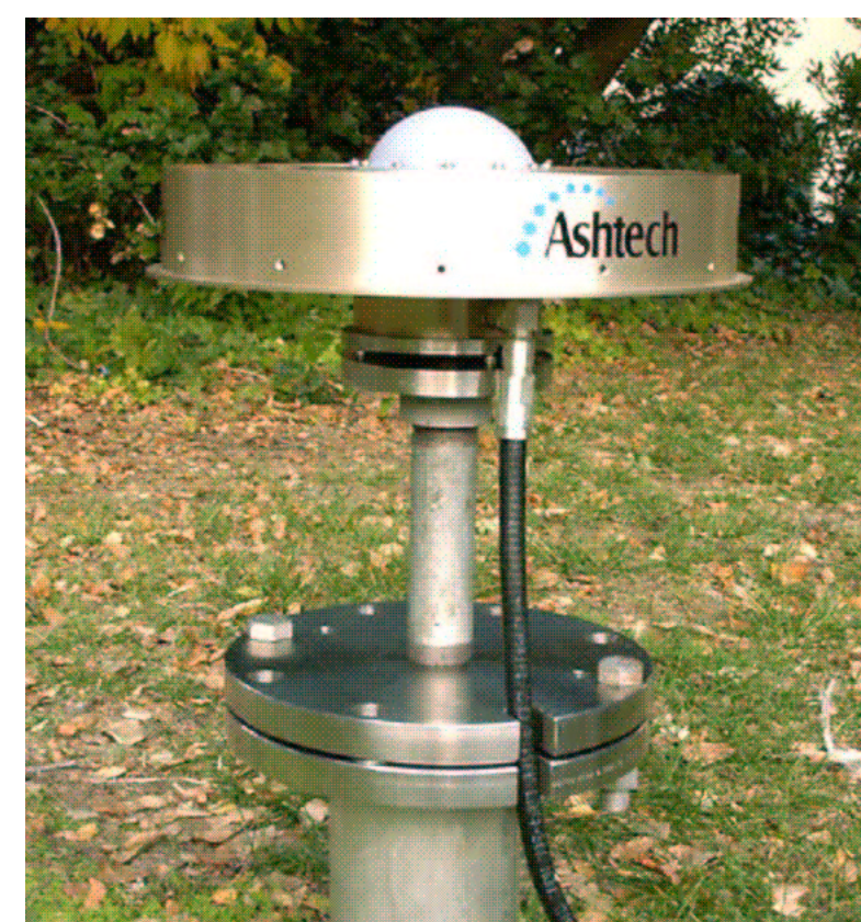
New GPS antenna mount design, using modified commercial flanges that enable high-precision self-center while allowing access to the top of the borehole for maintenance.
