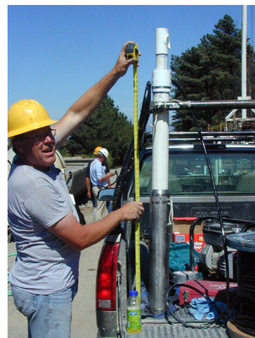
The 3-component seismometer package (Mark L22 velocity sensors) is readied for deployment at Marin Headlands.
