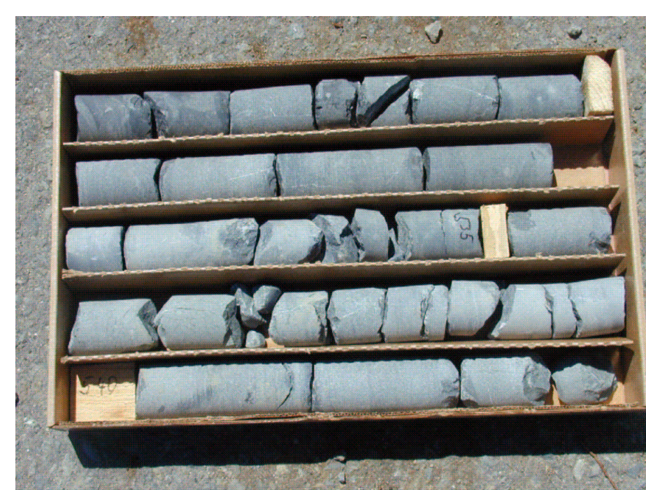
Cores recovery was generally poor. Visual inspection by camera was a more reliable method to assess the competence of the rock.
