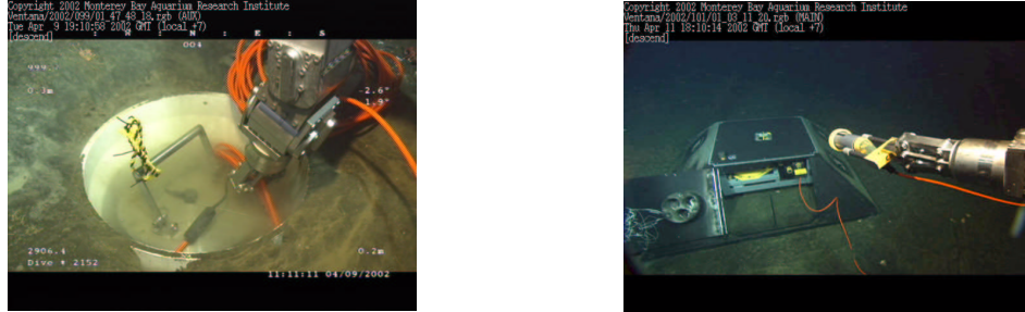
Figure 2: left: Installation of the seismometer package inside the PVC caisson. This was later completely covered by glass beads. Right: Trawl-resistant enclosure for the recording and battery packages. This snapshot was taken as the ROV Ventana was bringing the cable from the seismometer package in order to connect it onto the recording package. The first time such a remote underwater connection was attempted during the MOISE experiment, it took 2.5 hours to succeed and led to a redesign of the geometry of the instrument packages. The ROV operators are now able to do this routinely in less than 5-10mn.
