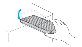
5. To clean any dust remaining on the air filter, use a small vacuum cleaner designed for computer and other office equipment to clean the front. If you don't have one, gently clean the vent with a soft brush (such as an artist's paintbrush).
