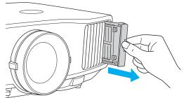
3. Place your finger into the groove and remove the air filter as shown.
