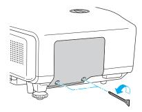
4. Loosen the two screws holding the lamp in place (you can't remove them).
