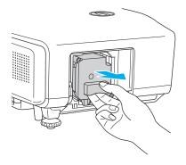
6. Gently insert the new lamp. (If it doesn't fit easily, make sure it is facing the right way.)
