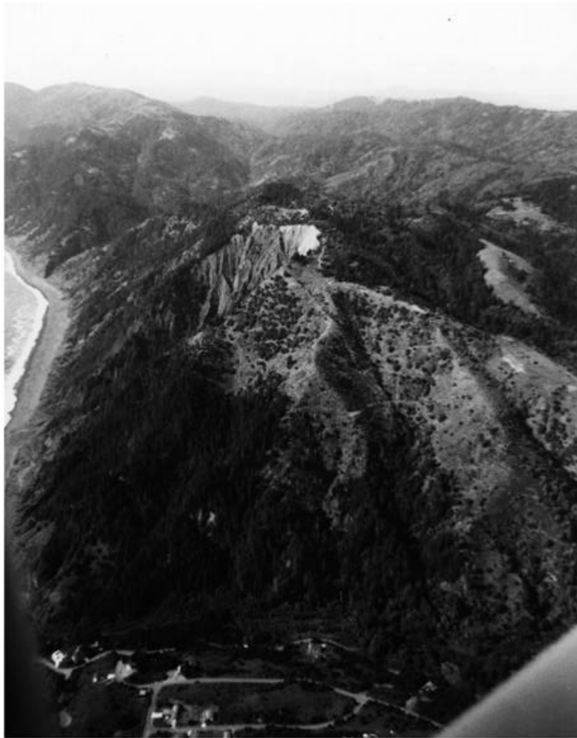
FIGURE 9. Right-lateral transform motion between the Pacific and North American plates produces slip along the San Andreas fault, coastal California. View to north of Telegraph Hill (T), at the northern termination of the San Andreas fault system. Note prominent east-facing scarp indicated by long, white arrows. Scarp diverges into two traces, marked by short, white arrows, near top of hill. Sense of motion on the main trace (westernmost scarp) is oblique, with both right-lateral and reverse (up to the west) motion. Kaluna Cliff (KC) is in middle ground. Prominent notch (N) along skyline marks northernmost feature identified as possibly related to Quaternary fault activity. Low-sun-angle oblique aerial view taken in June 1995 by photographer Cheryl Stolfus Shenk. ( From Prentice, Carol S., Merritts, Dorothy J., Beutner, Edward C., Bodin, Paul, Schill, Allison, and Muller, Jordan R., 1999, Northern San Andreas fault near Shelter Cove, California: GSAB , v. 111, no. 4, p. 512-523.)
