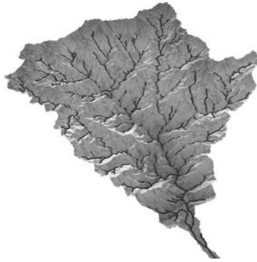
Figure 1 Perspective view of Haulien River basin (447 km 2 drainage area, 3580 m relief), Central Range, Taiwan. Channel network with minimum supporting first-order drainage area of 0.8 km 2 shown ( A > A_{cr} , see Equation 2). Eighty to 90% of topographic relief is on the channel network (Table 2).
