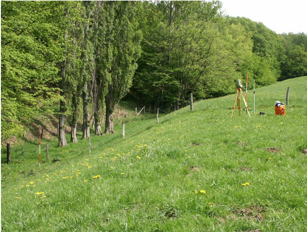
Figure 7.1. Data acquisition with a total station in the field. Profile 2 (Hausen). View to SE.
