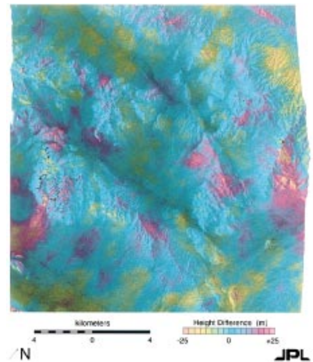
Fig. 35. Difference image between SIR-C C-band derived DEM and a TOPSAR mosaic used as a reference DEM.
