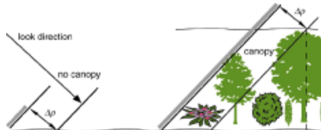
Fig. 22. A view of volumetric decorrelation in terms of the effective radiating ground resolution element, showing the increase in the size of the projected range resolution cell \Delta\rho_l (shaded boxes) as scattering from the volume contributes within a resolution cell.
