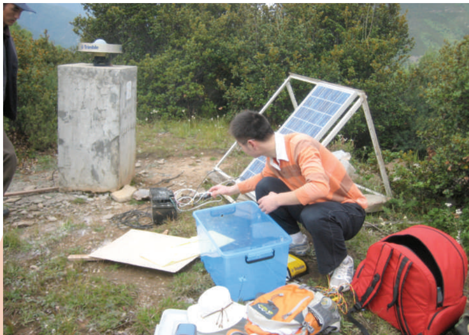
A crew member setting up GPS survey instruments at a mountain-top site after an hour-long hike. He is being watched by a local villager who helped carry survey equipment to the site.
