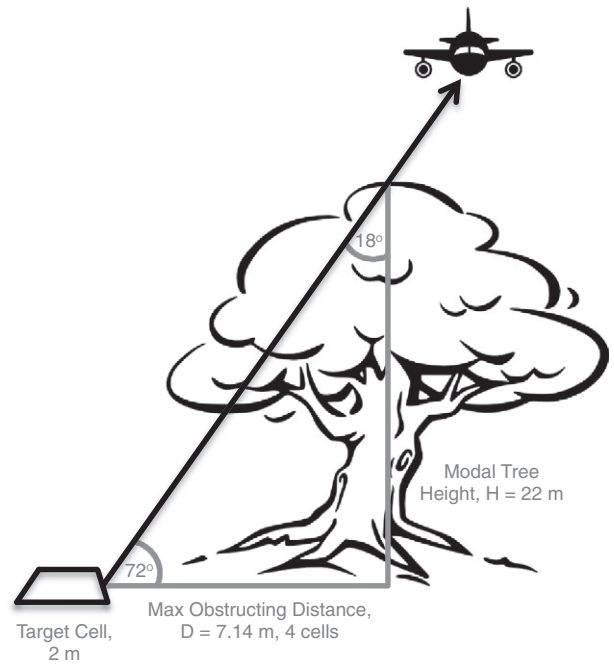
Fig. 7. Maximum obstructing distance of vegetation is a function of the height of the neighboring vegetation and the scan angle of the laser. For sunlight this would be infinite, since the sun sets at the horizon, but using the LiDAR scan angle provides a practical starting point.
