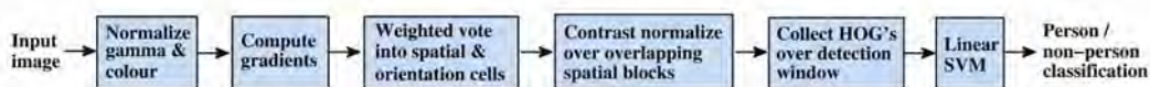
Figure 1. An overview of our feature extraction and object detection chain. The detector window is tiled with a grid of overlapping blocks in which Histogram of Oriented Gradient feature vectors are extracted. The combined vectors are fed to a linear SVM for object/non-object classification. The detection window is scanned across the image at all positions and scales, and conventional non-maximum suppression is run on the output pyramid to detect object instances, but this paper concentrates on the feature extraction process.
