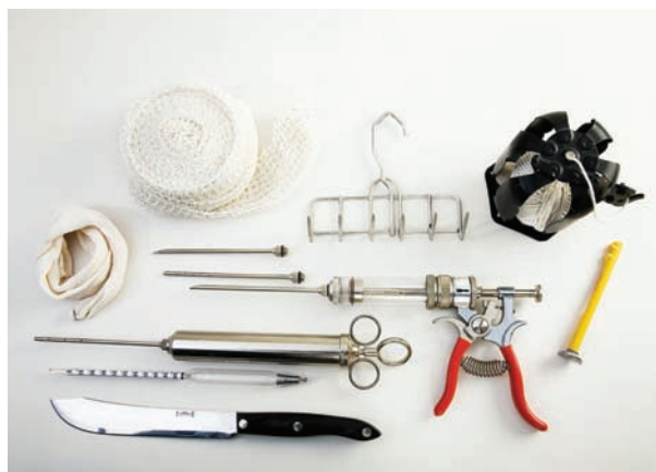
Top, left to right: Netting for hams, bacon holder, butcher twin. Second from top, left to right: Salami netting, needles for brine pump, large brine pump, hand thermometer. Middle row: simple brine pump. Second from bottom: salt meter. Bottom: butcher knife
