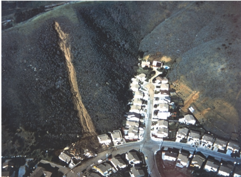
Figure 1.1. Shallow landslides in the San Francisco Bay area. a) Shallow landslides on hillslopes near Briones, California, showing a range of size and location (note that the unvegetated scars partly include the runout portion of the slide; scene width is about 300m), from [Dietrich, et al., 2008]. b) A landslide that struck Pacifica, CA, in 1982, destroying two residences and killing three children [photo: USGS].
