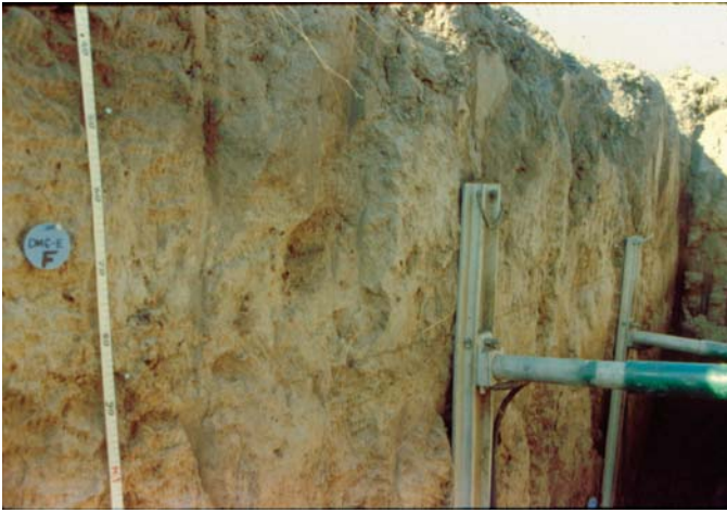
Figure 26. Light gray “E” horizon developed on the NE side of the Hayward fault in Trench DMG-E, a few meters from the soil profile in Figure 25 (Borchardt, 1988a).
