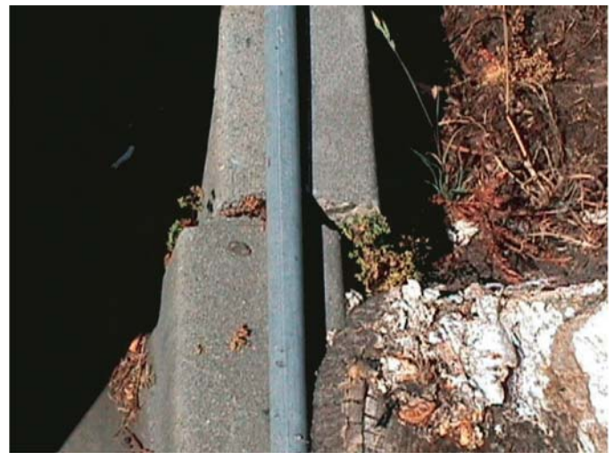
Figure 45. Photograph of evidence of right lateral creep on the mapped active strand of the Hayward fault. This offset curb is in the parking lot between A and B streets in downtown Hayward.
